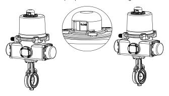
Remove valve mechanical stops and mount on the proper connection.
